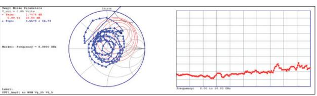
Wideband noise parameter measurement between 8 GHz and 50 GHz using PNA-X without additional NRM
