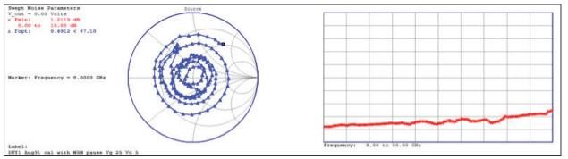
Wideband noise parameter measurement between 8 GHz and 50 GHz using PNA-X with additional NRM
