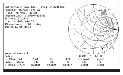
Figure 1. Power Added efficiency Contours vs. Second Harmonic Load Impedance.
