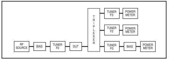
Figure 2. Load Pull Setup with Triplexer Load harmonic Tuning.
