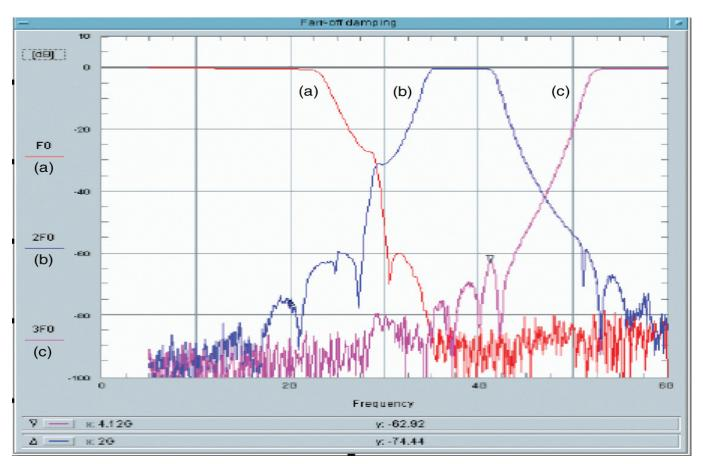
Figure 5. Typical Insertion Loss and Isolation of the Triplexer (a = Fundamental Path, b = 2nd Harmonic Path, c = 3rd Harmonic Path).
