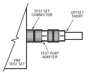
Figure 4. Set-up for Measuring Effective Source Match
