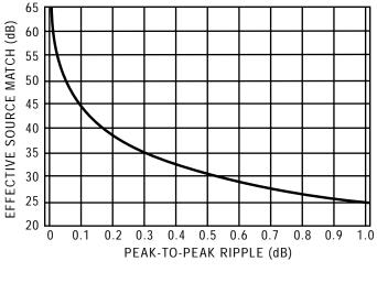
Figure 3. Plot of Effective Source Match Versus Peak-to-Peak Trace Ripple
