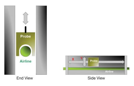
Figure 1. Simplified representation of a typical slide-screw tuner.
