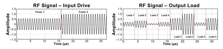
Figure 8. Injection signals as used in the "real-time" multi-dimensional parameter sweeps.
