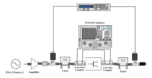
Figure 5. Vector-receiver load pull block diagram.
