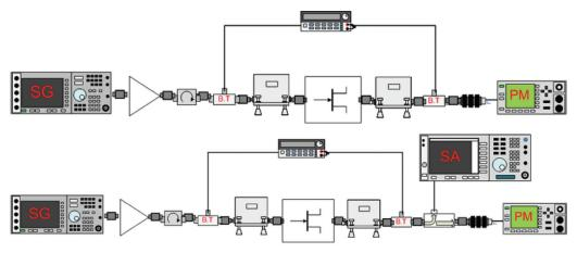
Figure 4. Traditional (scalar) load pull block diagrams.
