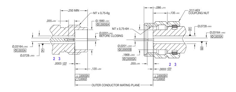
Figure 1. 1.85mm Connector Interface
