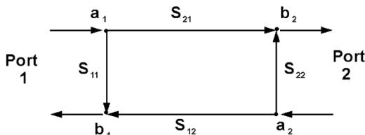
Figure 1. Two-port Scattering Parameter Model
