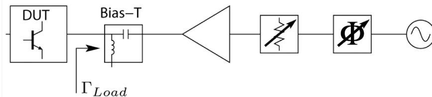
Figure 2. Open-Loop Active Tuning Block Diagram
