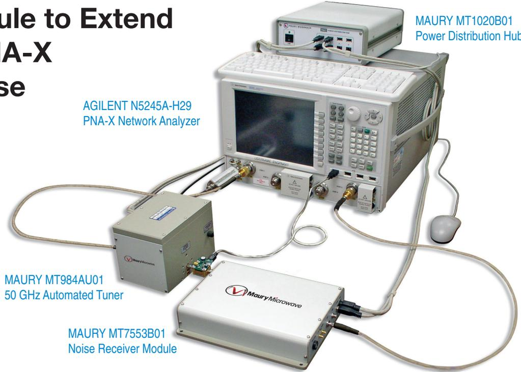
Typical setup for 8 – 50 GHz noise parameter measurements using a Maury MT7553B01 Noise Receiver Module and a Maury MT984AU01 Automated Tuner with the Agilent's PNA-X.
