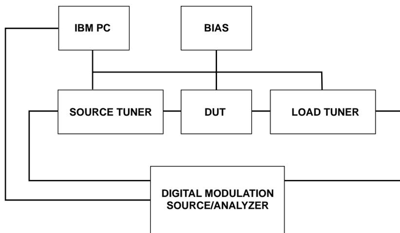
**Figure 1:** Diagram of the automated large-signal load-pull system.
