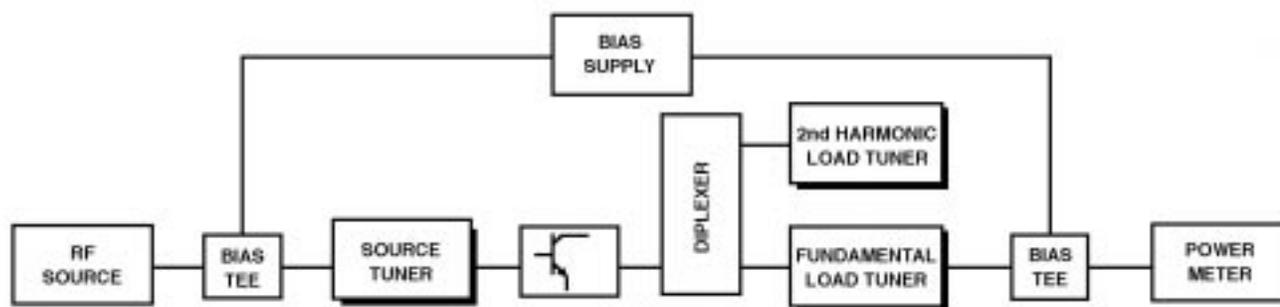
**Figure 2:** Basic Power Measurement Setup with 2nd Harmonic Load Tuning.
