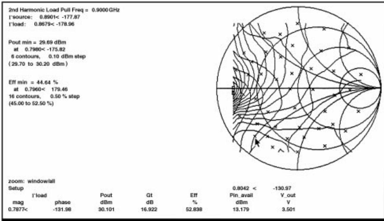
Figure 5: Contours of Constant Output Power and Efficiency vs. Harmonic Load Tuning (source and load power matched at fundamental).
