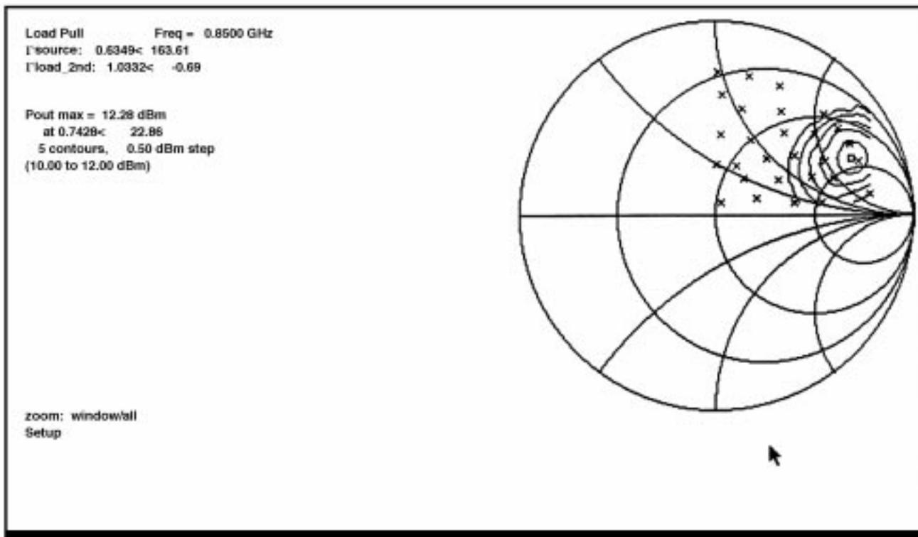
Figure 3: Contours of Constant Output Power at the Fundamental Frequency.
