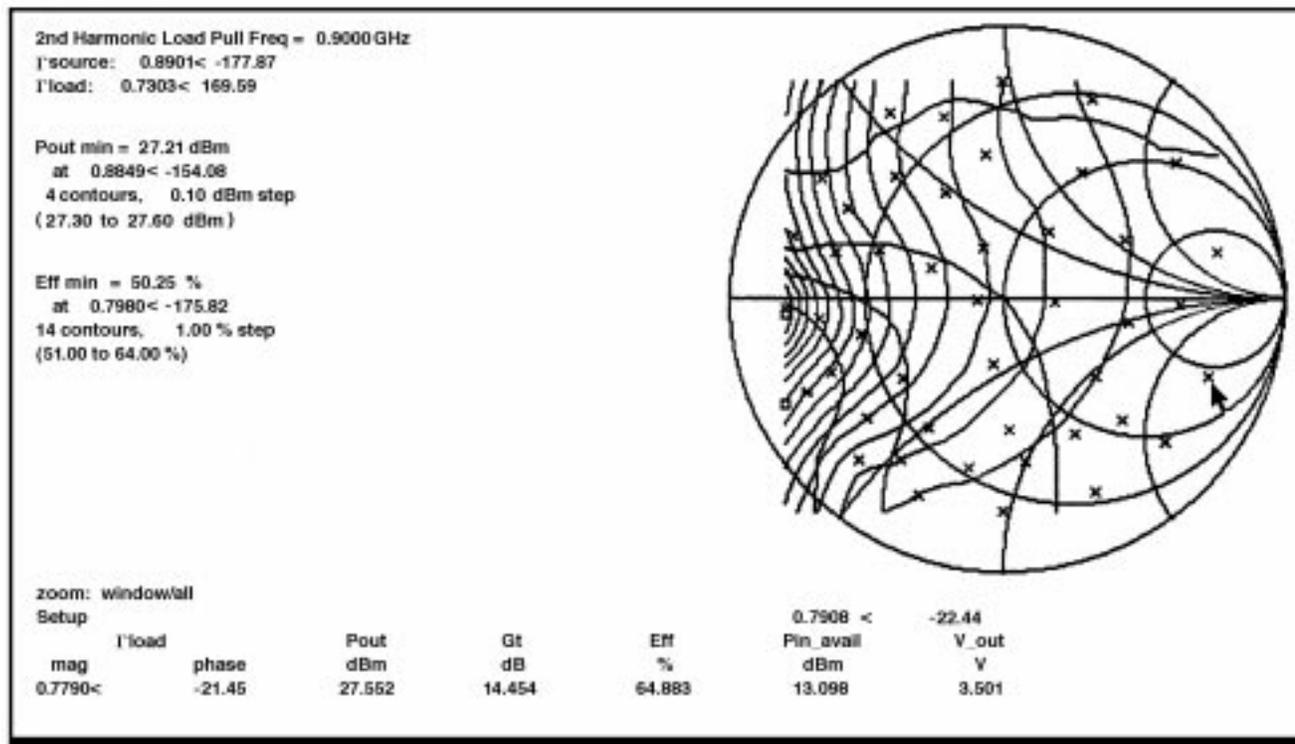
Figure 6: Contours of Constant Output Power and Efficiency vs. Harmonic Load Tuning (source power matched and load efficiency matched at fundamental).
