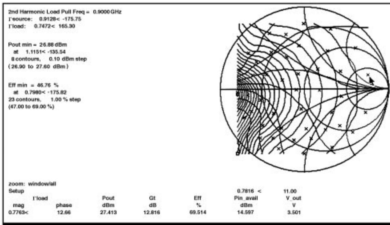
Figure 7: Contours of Constant Output Power and Efficiency vs. Harmonic Load Tuning (same as Figure 6, except slightly higher input power).
