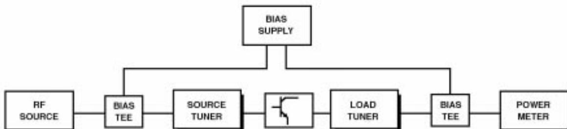
**Figure 1:** Basic Power Measurement Setup with Tuners.
