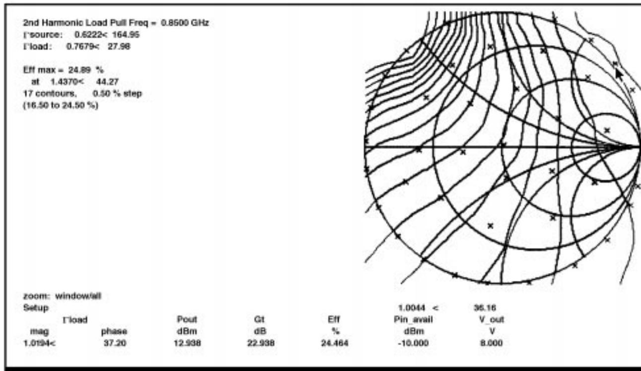
Figure 4: Contours of Constant Efficiency vs. Harmonic Load Tuning.
