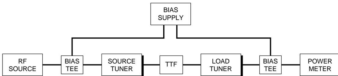
Figure 1: Passive Tuner System for Basic Power Measurements
