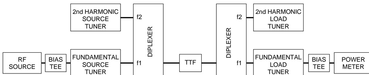
Figure 2: Passive Tuner System with 2nd Harmonic Source and Load Tuning
