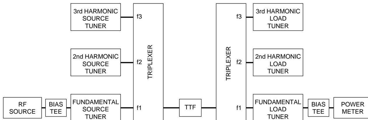
Figure 3: Passive Tuner System with 2nd and 3rd Harmonic Source and Load Tuning
