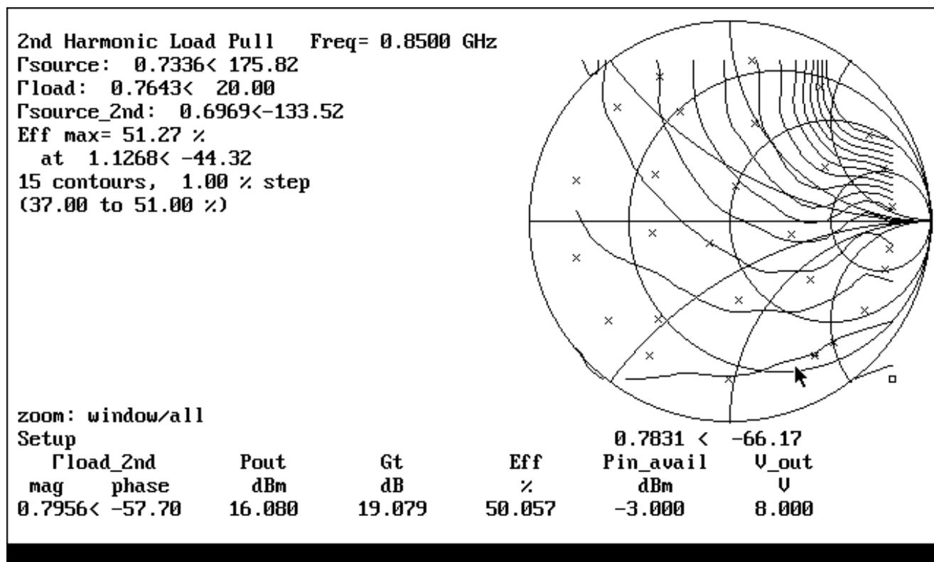
Figure 4: Efficiency vs. 2nd Harmonic Load Tuning
