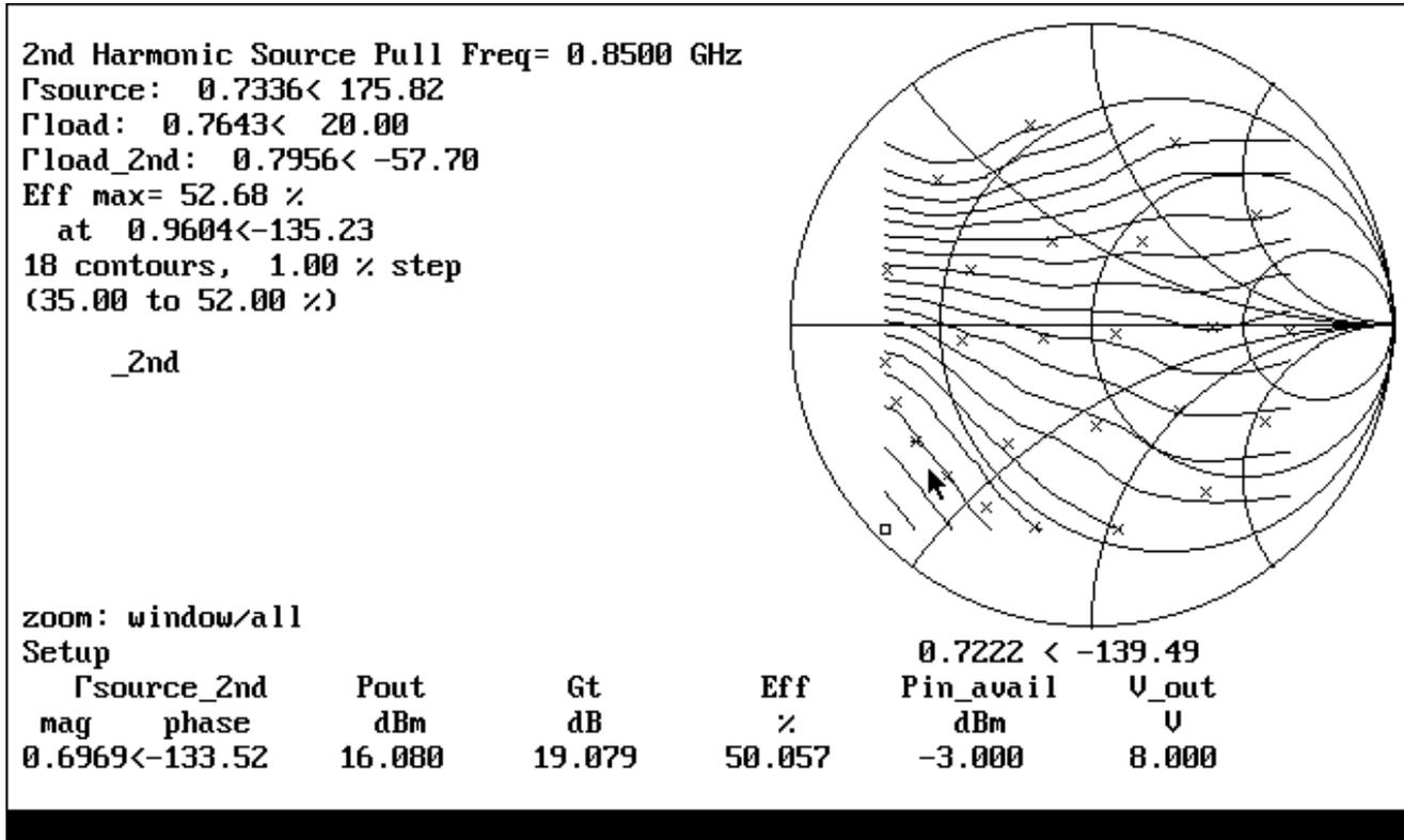
Figure 5: Efficiency vs. 2nd Harmonic Source Tuning
