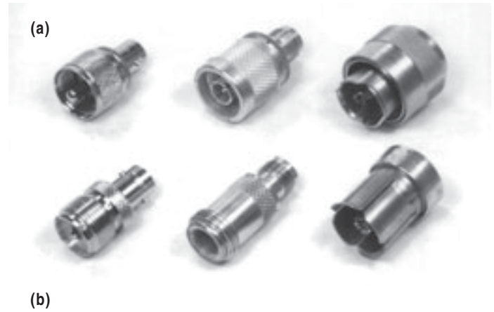
Figure 3: Early coaxial connectors; UHF female and male adapters to BNC female, MIL-C-71 type N connectors female and male adapters to TNC female and GR874 connectors; (a) with and (b) without locking nut.
