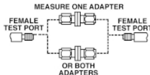
**Figure 4(b):** Extending the LRL technique for changing test port sex.
