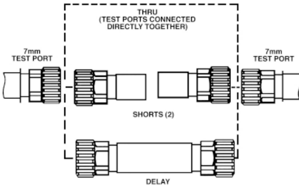
**Figure 3:** TSD calibration procedure using 7mm connectors.
