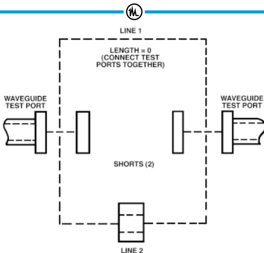
Figure 6: Basic LRL calibration in waveguide.
