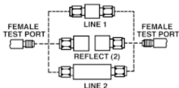
**Figure 4(a):** Basic LRL calibration procedure.
