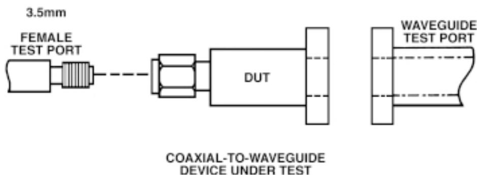
Figure 7: Measurement after two-stage LRL calibration.
