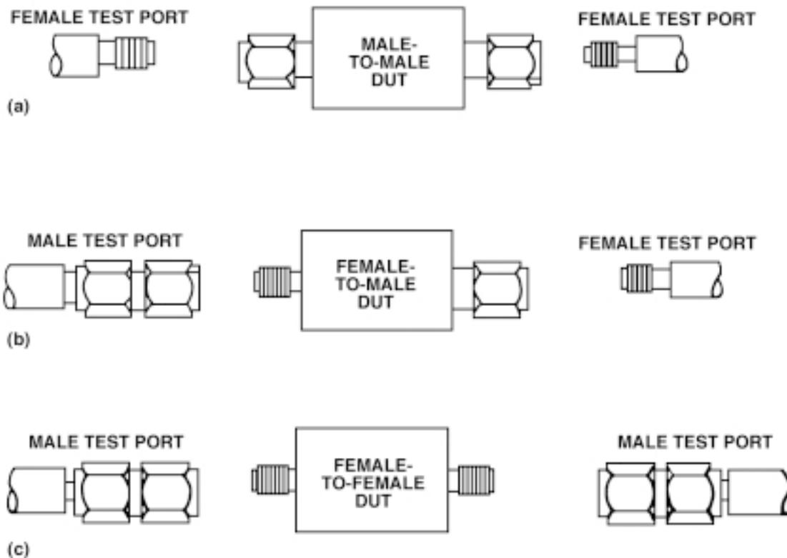
**Figure 5:** Measuring a DUT after LRL calibration and adapter measurement: (a) male-to-male DUT; (b) female-to-male DUT; (c) female-to-female DUT.
