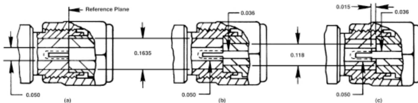
**Figure 5:** The "conventional" SMA connector achieves coplanar mating with the SMA female (a), but the "thru" male produces a capacitive discontinuity (b). Offsetting the female contact (c) can compensate for the mismatch.
