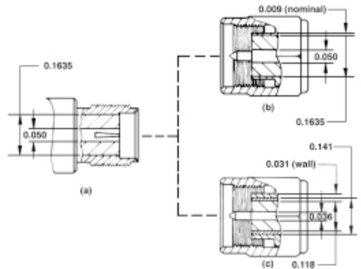
**Figure 1:** The single SMA female configuration (a) can mate with both the "conventional" male (b), and the "thru" male (c).
