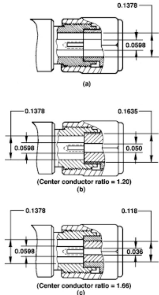
**Figure 3:** An APC3.5 mated pair (a) provides a precision junction with no discontinuities. Line size discontinuities are apparent when the APC3.5 mates to a "conventional" SMA connector (b), and are more of a problem with the SMA "thru" male (c).
