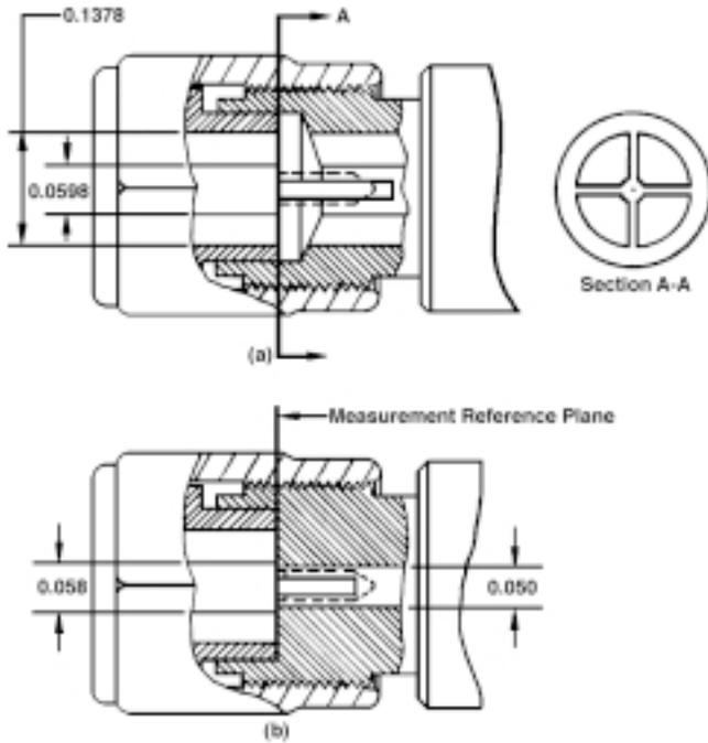
**Figure 9:** The design of the new reference plane female fixed short (a) is shown with an older "OSM" device (b). Section A-A depicts the radial slots in the face of the female contact which allow it to grab the male pin and make an almost perfect short circuit. The contact is made of beryllium copper, which is heat treated and gold plated.
