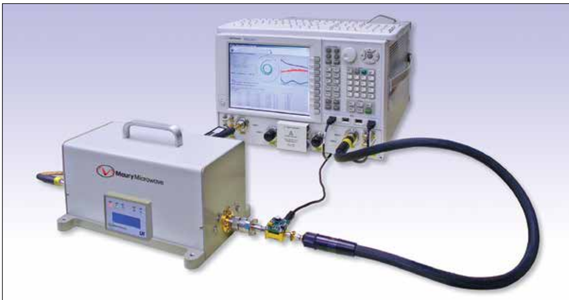
Typical setup for performing high speed noise parameter measurements.
