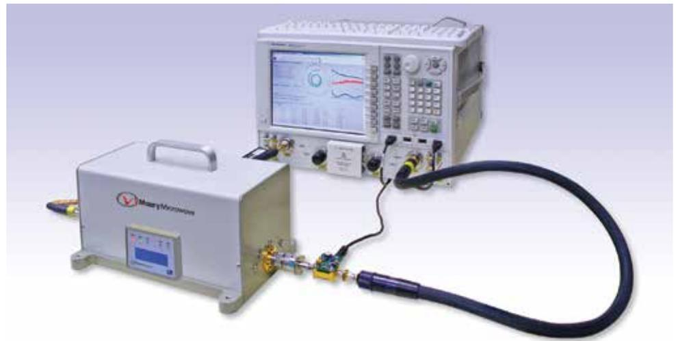
*Typical setup for performing high speed noise parameter measurements.*
