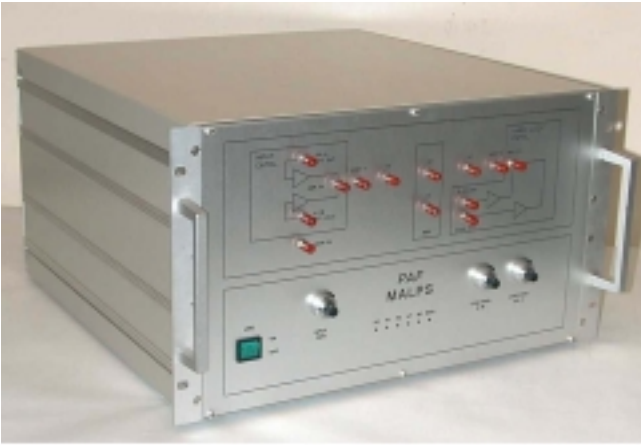
Figure 3. Two-loop active load unit.
