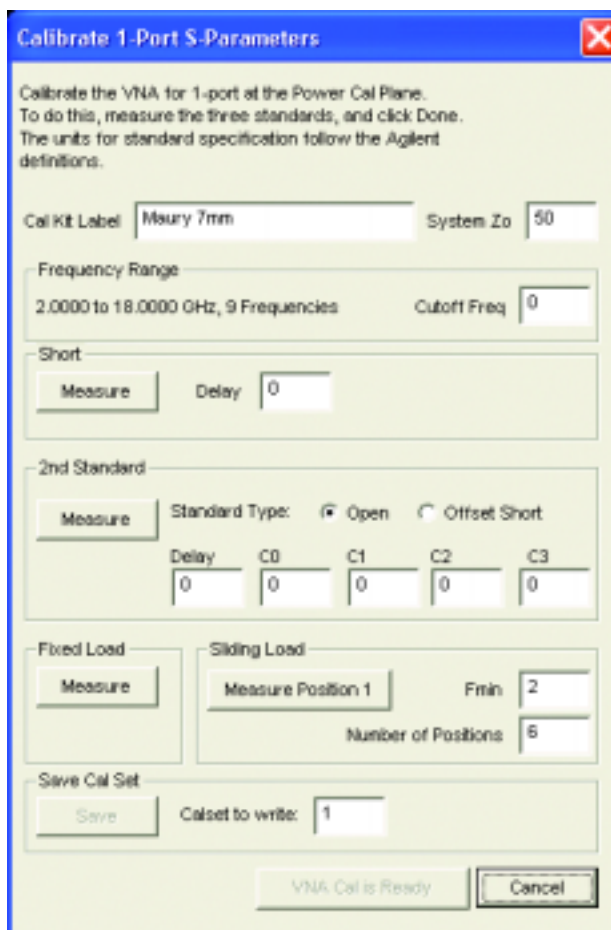
Figure 6b. Dialog Box Perform New VNA Calibration. Note That All Units Entered Follow Standard Agilent Definitions.
