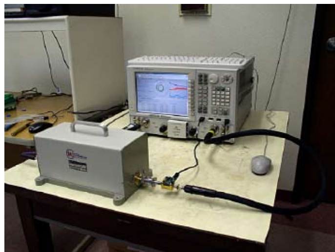
Figure 4. Photo of the new setup with the coaxial DUT.
