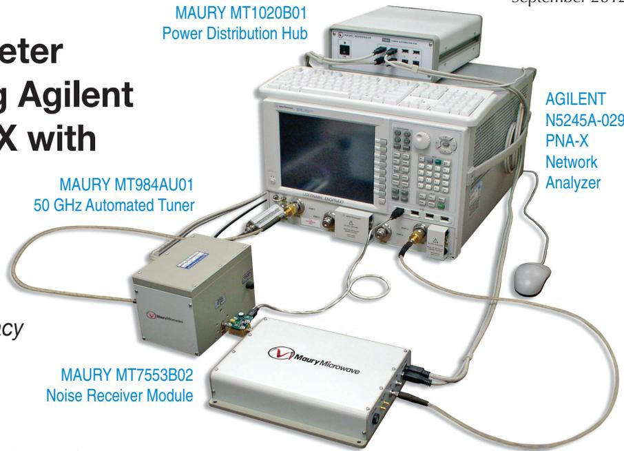
Typical 8–50 GHz noise parameter measurement setup using a Maury MT7553B02 Noise Receiver Module, a Maury MT984AU01 Automated Tuner and Agilent's PNA-X.
