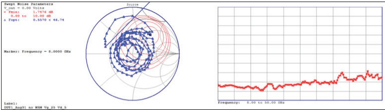
Wideband noise parameter measurement between 8 GHz and 50 GHz using PNA-X **without** additional NRM
