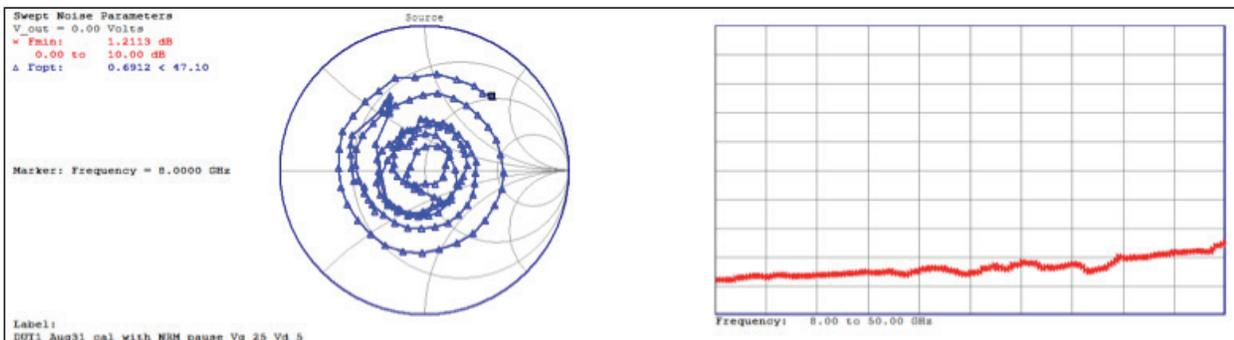
Wideband noise parameter measurement between 8 GHz and 50 GHz using PNA-X **with** additional NRM
