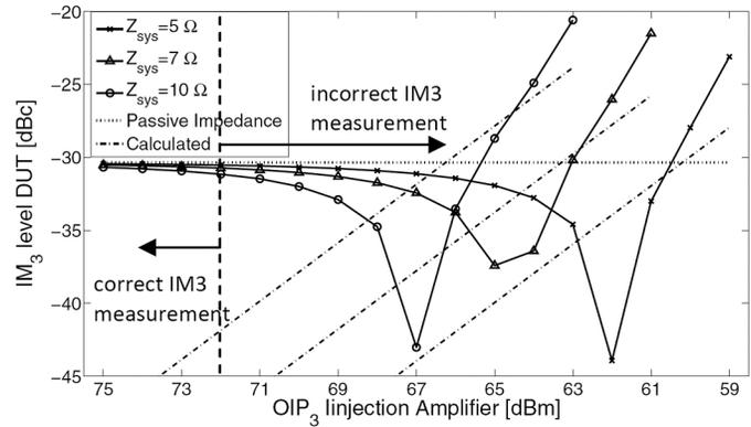
Figure 2. Harmonic balance simulated IM3 level of the DUT vs. decreasing output  $IP_3$  of the injection amplifier for different impedance pre-match values. The dotted line is the actual IM3 level as would be achieved with passive matching techniques. The dot-dash line represents the IM3 level due to the  $P_{a2,IM3}$  as approximated by Eq. (1). A polynomial model was used for the amplifier linearity.
