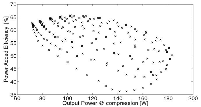
Figure 5. Measured PAE vs. output power at 3 dB power gain compression level of a NXP Gen7 LDMOS device for different load states and input powers, using pulsed single tone conditions (10  $\mu$ s pulse width and 10 % duty cycle).
